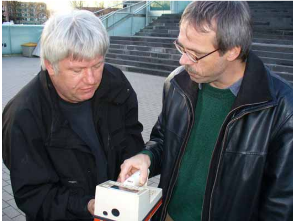
Testing the \alpha detector before driving to the site
