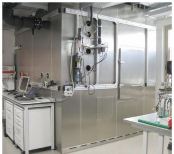
Example: BfS radon calibration chamber (11 m³)
