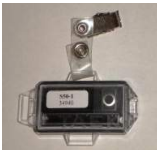
Figure 1: Example of a dosimeter with the label added by the coordinator. “S50” is the code to identify the dosimetry system (note: for presentation of the results, a different code was used). “1” is the code to identify a specific radiation quality, angle and dose range combination from the irradiation plan. 34940 is the participant’s own identification number.
