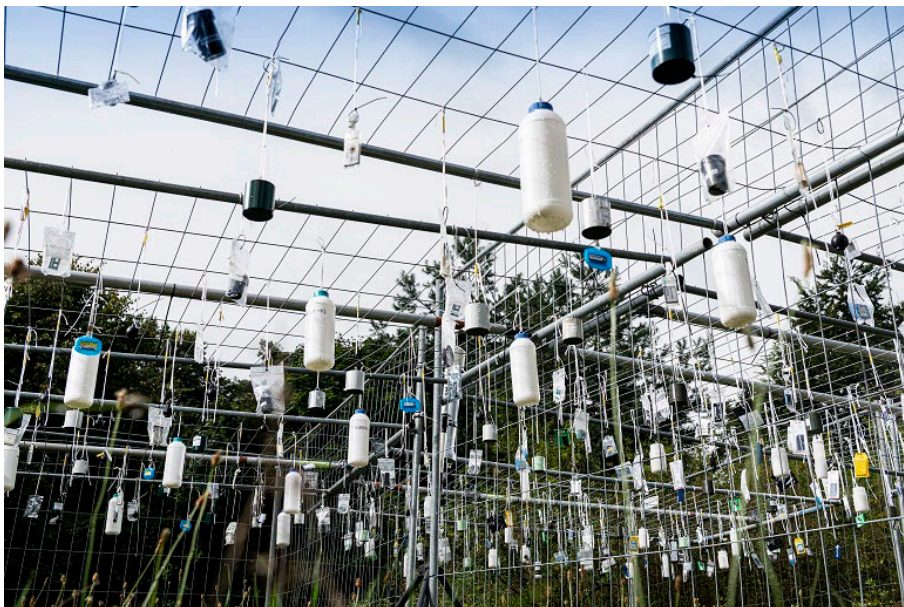
Figure 4.2: Dosimeters positioned on the outdoor measurement site at about 1 m height. Several dosimeter systems had no hanging possibility and were put into plastic bags which were not watertight.
